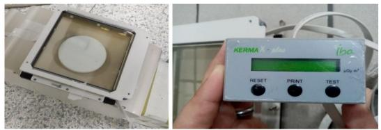
Figure 1. DAP meter used to measure DAP values (KermaX plus SDP, manufactured by IBA, Germany)
