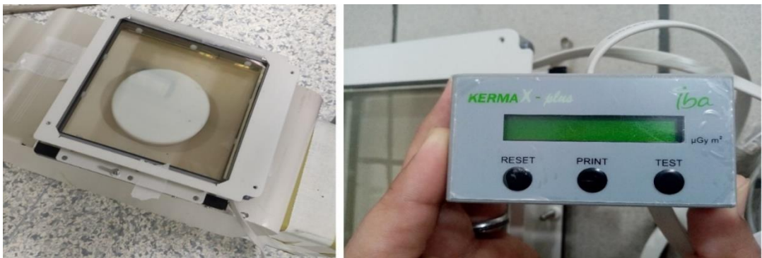
Figure 1. DAP meter used to measure DAP values (KermaX plus SDP, manufactured by IBA, Germany)
